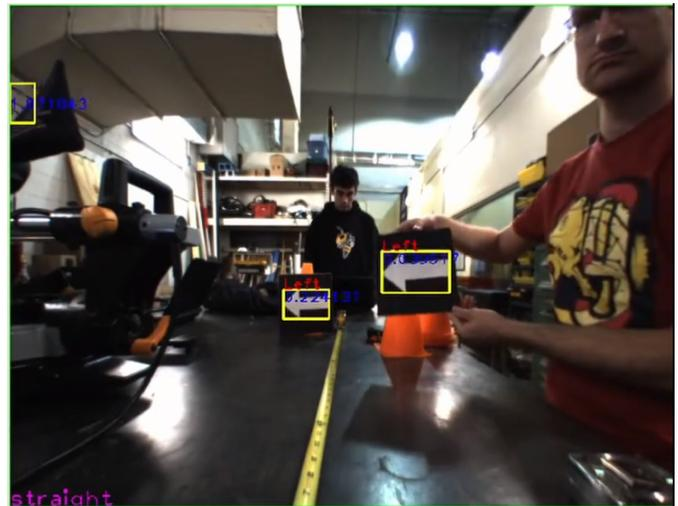
Fig. 9. Sign detector testing with multiple candidate signs in the image
