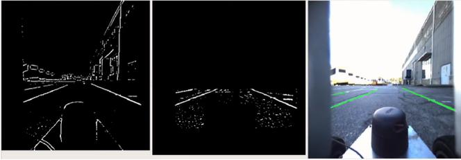
Fig. 8. Progression of lane detection operations, resulting in the green overlay of detected lanes on the far right image
